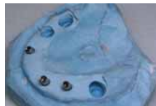
Fig. 6: Master cast with all ill-fitting replicas removed.
