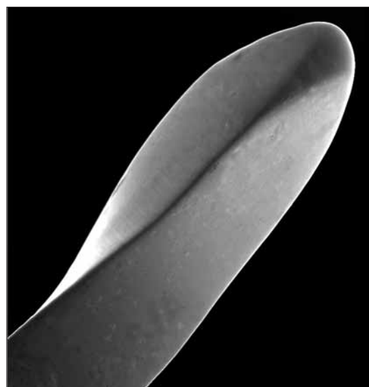
Fig. 2 The tip of an EndoSequence file after electropolishing.
